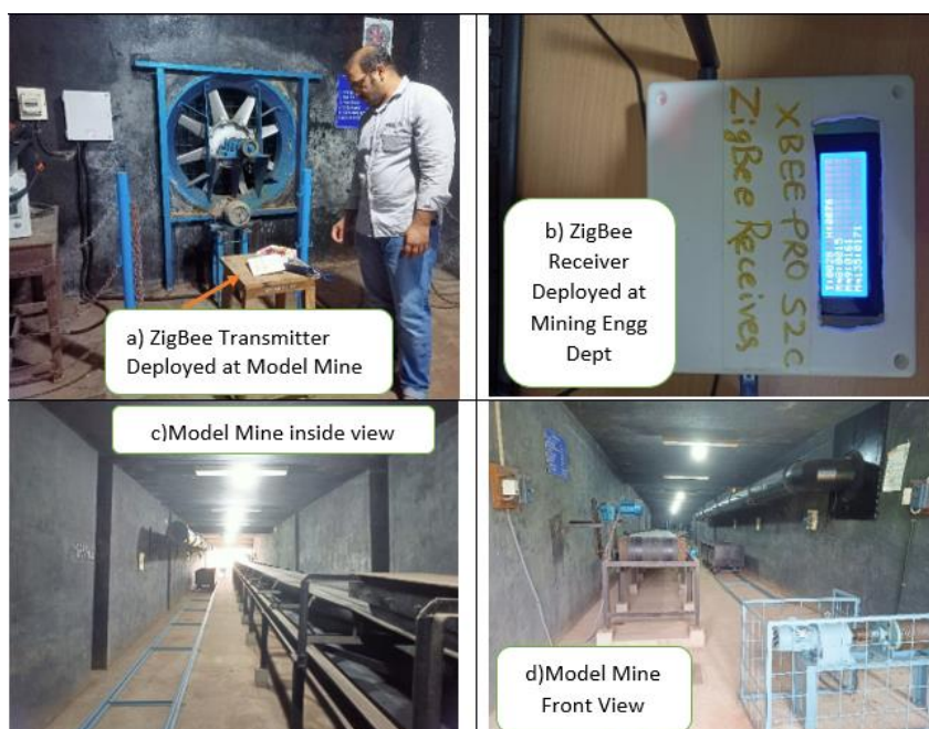
Figure 5: Deployment of Transmitter ZigBee Module in a model mine and Receiver at the Mining Engineering Department, NITK Surathkal. a) ZigBee transmitter deployed at model mine, b) ZigBee receiver deployed at the mining engineering department, c) Inside view of model mine, d) Front view of model view
