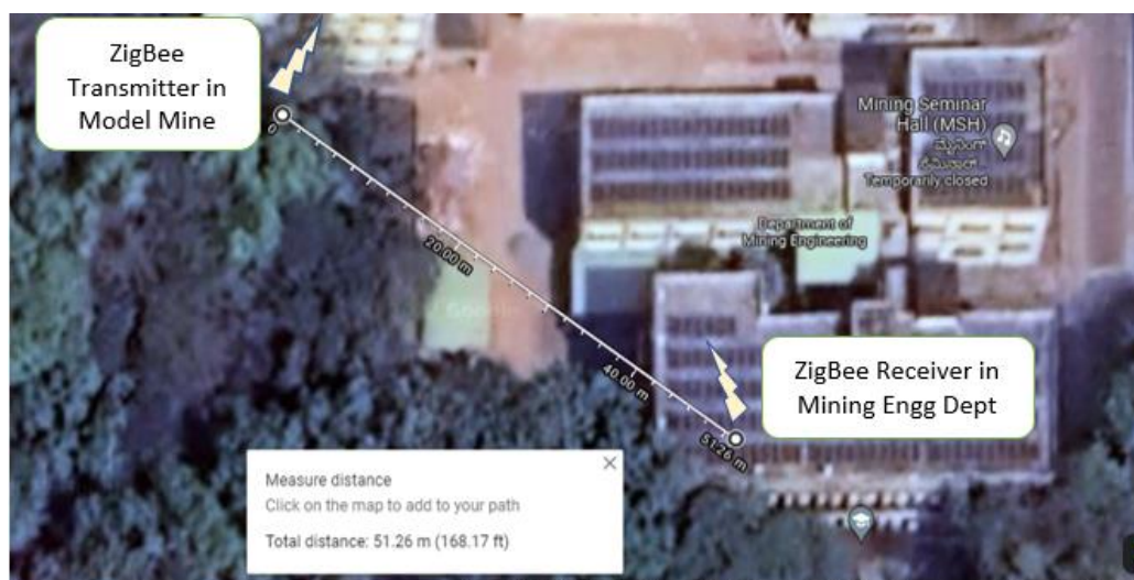
Figure 6: Deployment of the Transmitter ZigBee Module in a model mine and Receiver at the Mining Engineering Department, NITK Surathkal is represented as in a Google map
